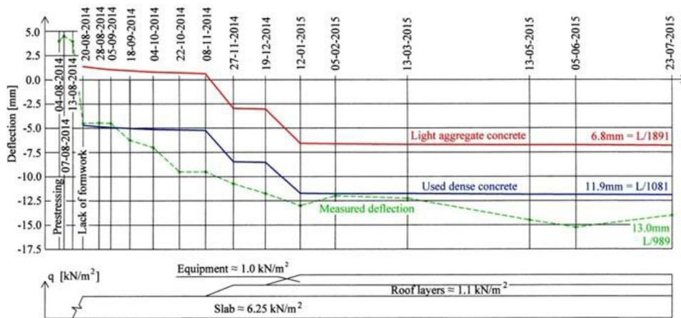
Fig. 8. Development of calculated and measured deflection.
