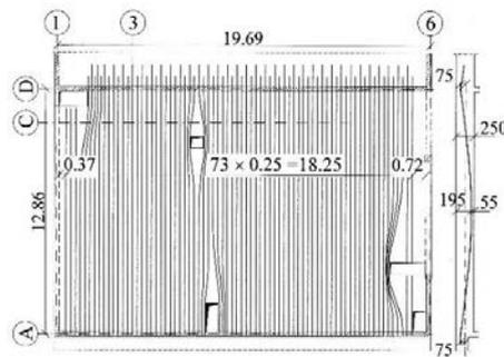
Fig. 4. Geometry and prestress arrangement of SI-2 slab.
